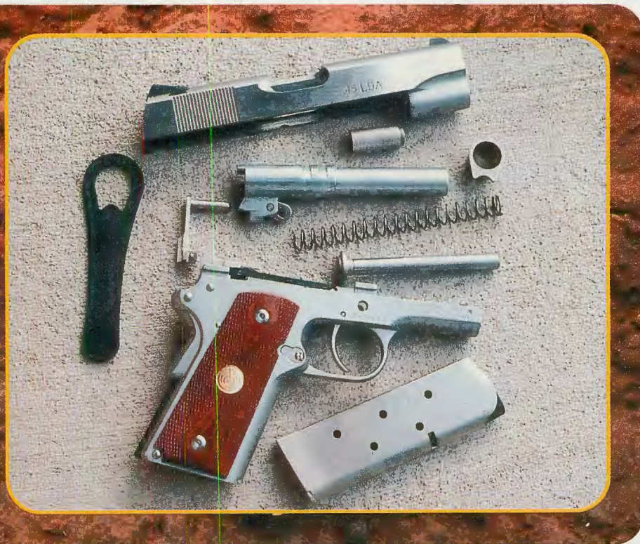
Disassembly was pretty much a cinch using just the polymer bushing wrench supplied with each gun.
